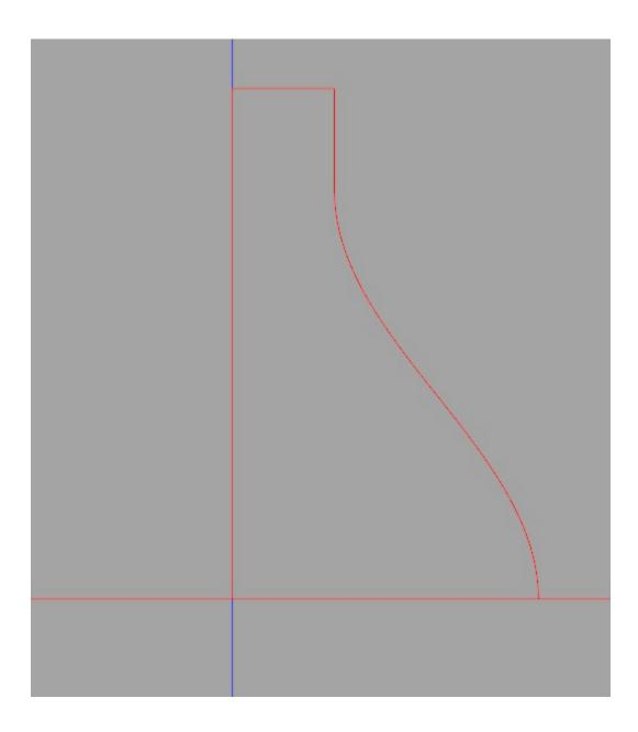
The revolve function is used after that on this 2D sketch, and takes as variables axisstart and axisend, to make sure that the rotation will be around the Z axis, and takes also a boolean variable: clean set to True, to clean the 2D sketch. As a result we get the following.
